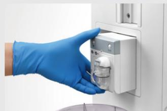
Mindray Plug-and-Play Multi-Gas modules provide comprehensive breath-by-breath analysis of O<sub>2</sub>, CO<sub>2</sub>, N<sub>2</sub>O, and auto-detection of five anesthetic agents, as well as BIS.
